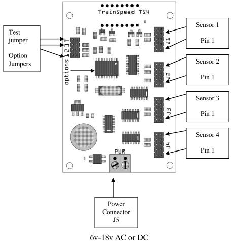
Input polarity does not matter
